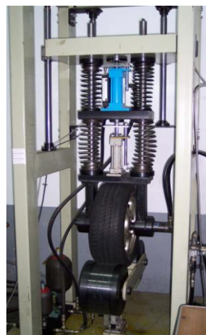
Figure 1 Hydraulic actuating quarter-car active suspension system
